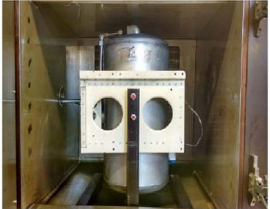
Fatigue Testing is carried out with the objective of determining the relationship between the stress range and the number of times it can be applied before causing failure.
