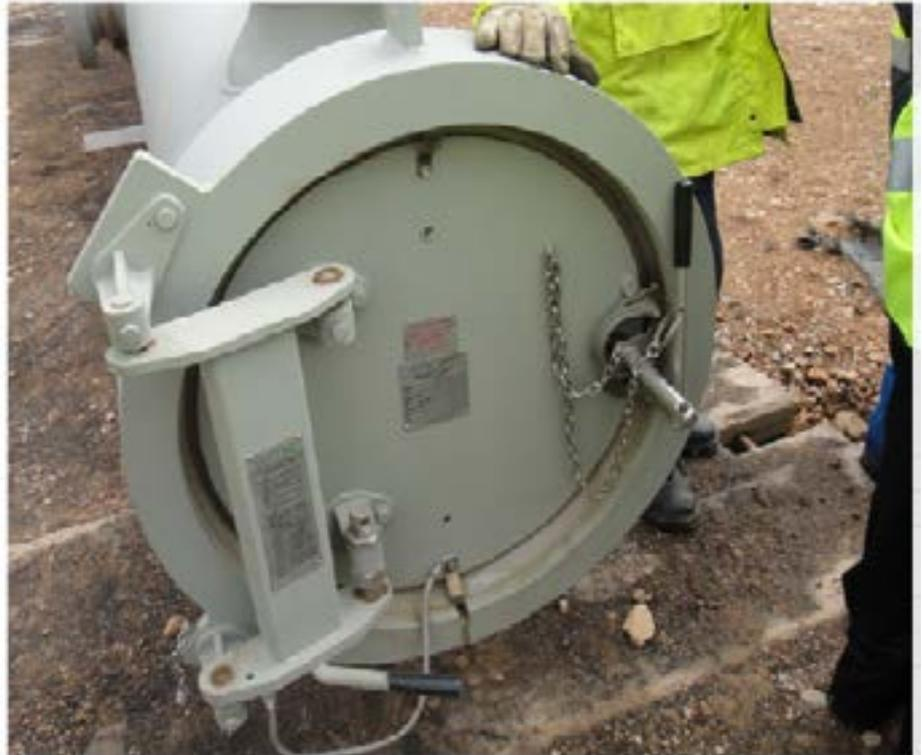
Pipeline Inspection Gauges (PIGs) are essential for National Grid to monitor the integrity of its transmission network - to ensure it is safe, secure and fit for purpose.
